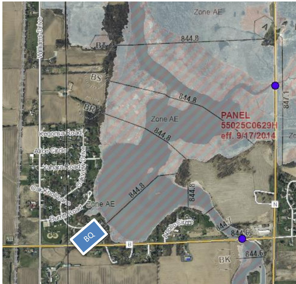
Figure 4. Location of cross section BQ in the widening upstream of CTH B (from WDNR Surface Water Data Viewer). Shaded and hatched patterns show 100-yr floodplain and floodway, respectively.
